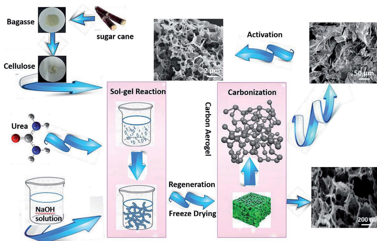
Figure 23. Schematic of the fabrication of highly porous bagasse-derived carbon aerogels with hierarchical pore structure according to Hao et al. 149 Reprinted with permission from Nanoscale, Copyright (2014) Royal Society of Chemistry
