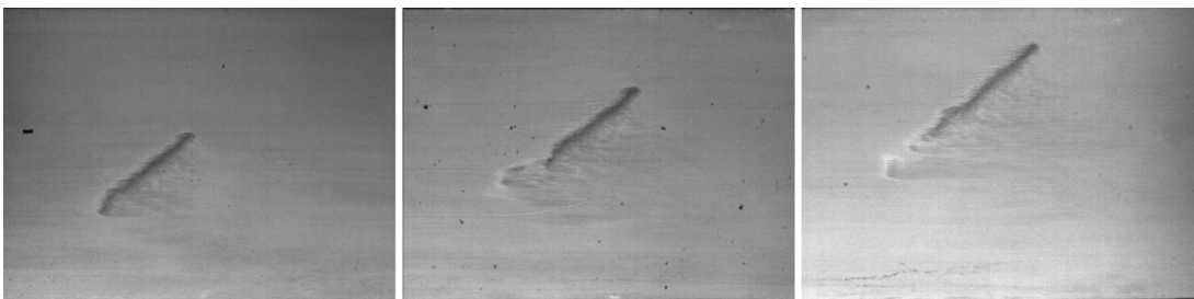
Figure 3.10: Growing turbulent stripe at Re = 675 . When a continuous addition of new streaks at the downstream tip is more than an intermittent streak decay at the upstream tail, the stripe length increases in an average sense as it is advected in the streamwise and spanwise direction. The flow is from left to right.
