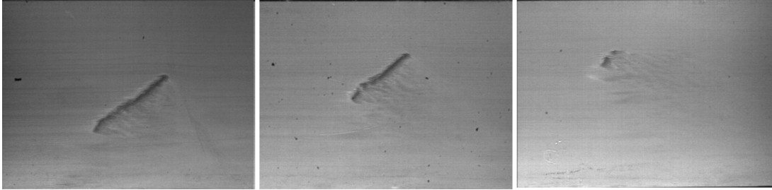
Figure 3.9: Decaying turbulent stripe at Re = 640 . The stripe grows at the downstream tip by adding new streaks and decays from the upstream tail by shedding streaks. When the shedding rate at the tail is higher than the addition of new streaks from the tip, then the result is an eventual decay of the stripe. The flow is from the left to the right.
