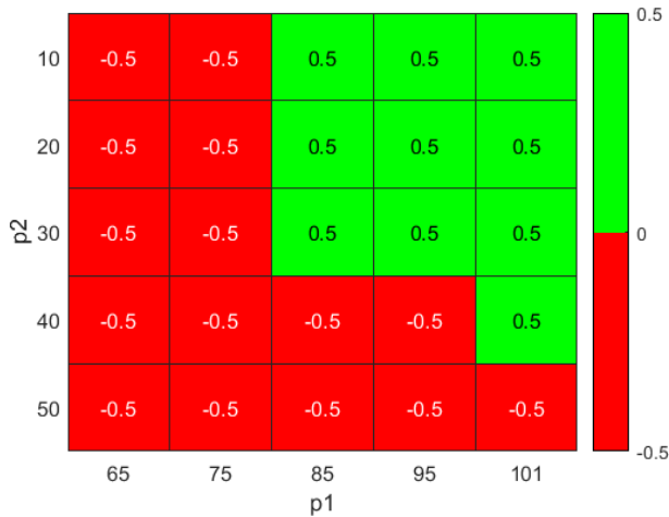
Figure 8: Heatmap for the Fuel Cell system, requirement R and p_3 = 90 , using classical STL robustness computation.
