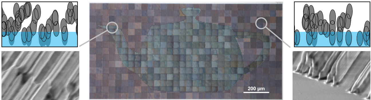
Fig. 1. (Center) Microscope image of a structurally colored surface with the corresponding nanostructures of the fore- and background depicted left and right of it. (Top) The cross-sectional profiles of both transparent structures were designed with our method using full electromagnetic simulation. (Bottom) Micrographs of the fabricated nanostructures with a length scale of 5 \mu\text{m} across the image diagonal.
