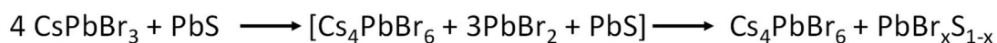
Figure 2.1.1. Chemical transformation of CsPbBr 3 into Cs 4 PbBr 6 triggered by the dissolution of PbBr 2 in PbS.
