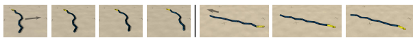
Figure 1: Side-rolling and crawling of the SNAKE. The segments are linked with 2-way hinge joints.
