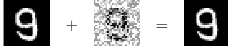
Figure 2.1: Illustration of an adversarial attack on a 8-bit quantized neural network trained on the MNIST dataset. The image of the left is correctly classified as the digit "9", whereas the image of the right is misclassified as "3".
