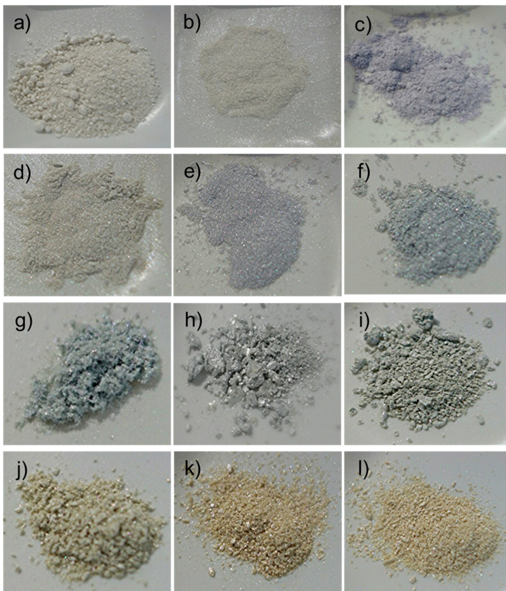
Figure 2. Color variation of CPs depending on the deposition pH; (a) Mica flakes, (b) MT, (c) CP deposited at ACN extraction pH (i.e., 4.37), CPs deposited at pH values of (d) 2, (e) 3, (f) 4, (g) 5, (h) 6, (i) 7, (j) 8, (k) 9, and (l) 10.
